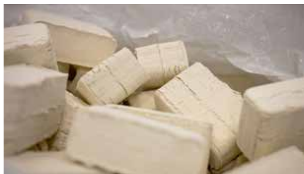
Polyurethane dust collection from saw lines and briquetting
