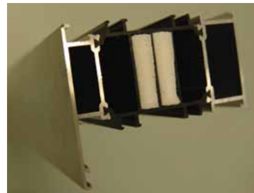
➤ Innovative 'smart' foam for use in hollow aluminum window profiles.
